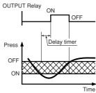
\*In case pressure increase than the ON pressure during working of Delay timer, timer is reset, and dose not turn on.
